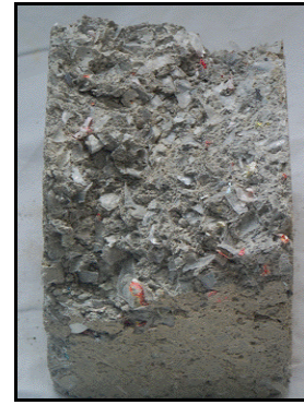
Fig 3: Cross section through PET block after Compression Test.
