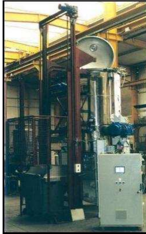
Figure 6: Photograph showing a T2000 ECODAS Steam Sterilization and Shredding Treatment Equipment (Source: SEEN Environnement 2006)
